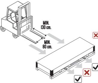
To handle them by their wide part we recommend using forks of at least 130 cm in length and a forklift truck of minimum weight 2,000 kg. The minimum distance between blades is 80 cm.
