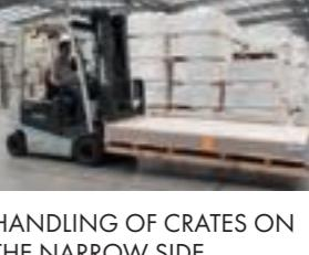
When handling the crate lengthwise it is recommended to use forks of at least 240 cm and a forklift truck of minimum weight 2,000 kg. The minimum distance between forks is 80 cm.
